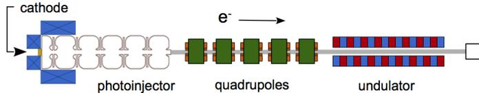
Figure 1: Layout of the accelerator showing the 5.5-cell photoinjector with its bucking coil and solenoid, the cathode, the quadrupoles, the undulator, and the beam dump.
