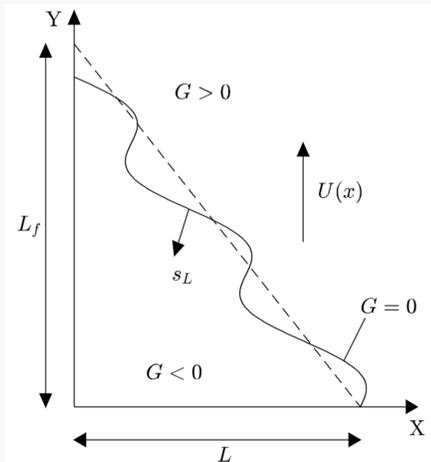
The G-equation is a kinematic reduced-order model that describes flame response to acoustics. It models the flame as an infinitely-thin front propagating into unburnt gases at a fixed speed  $s_L$ . The flame front is defined as the  $G = 0$  contour of the two-dimensional time-varying G-field  $G(x, y, t)$ .
