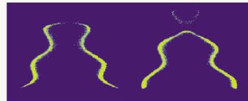
Experiments were performed at different fuel compositions (methane: ethene ratios), flow rates, excitation frequencies (250 - 450 Hz) and excitation amplitudes.
