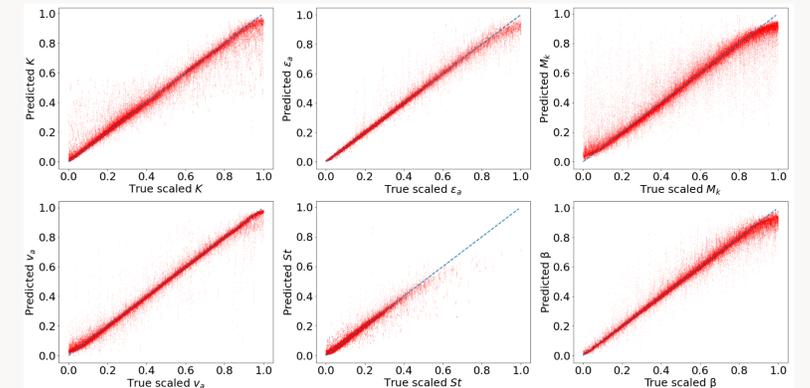
We use the trained network to predict parameter values for 10 experimental flame videos and re-simulate the flames using predicted parameter estimates. The re-simulated flames match the dynamics of the real flames closely.
