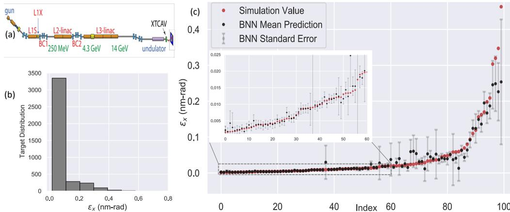
Figure 2: A) Schematic of the LCLS Beamline, b) Distribution of target emittance ( $\epsilon_x$ ) in the learning data sampled uniformly in feature space, c) BNN mean predictions and standard errors for a sample from the test set, with an inset view of the lower ranges.
