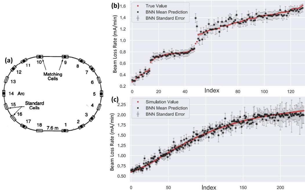
Figure 1: (a) Schematic of SPEAR3 Ring, BNN mean predictions and predicted standard error for (b) SPEAR3 measurements, (c) simulation data. Here we sort the simulation values by magnitude and show corresponding predictions. The beam loss rate is a proxy measure for the beam emittance.
