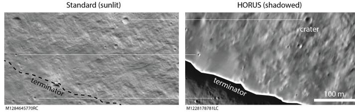
Figure 4: Ground truth verification. The comparison of a non-HORUS sunlit and a HORUS shadowed image (contrast and brightness-adapted) in a temporarily shadowed region indicates that our denoising does not remove or add any physical features. Non-HORUS image credit to LROC/ASU/GSFC.
