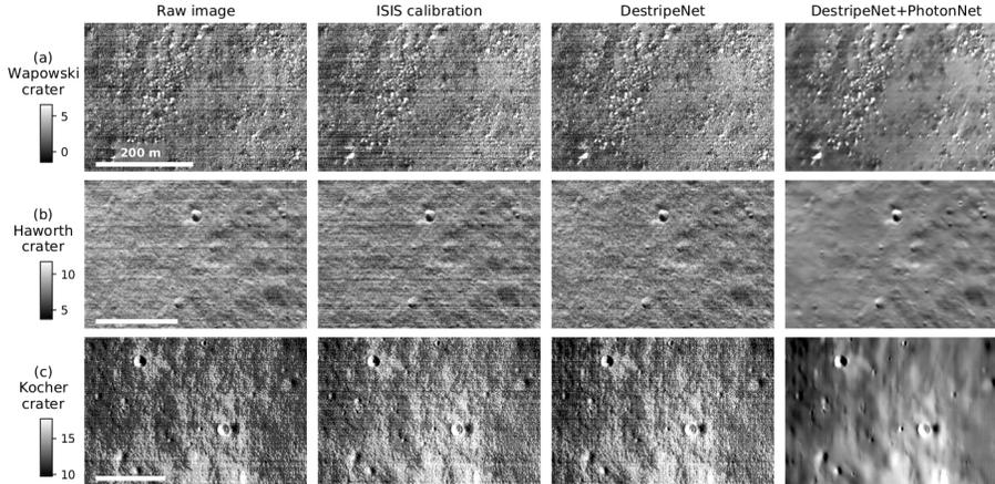
Figure 1: Performance of HORUS over 3 example PSRs, compared to the current calibration routine (ISIS) (Humm et al., 2016; Gaddis et al., 1997). Colour bar shows the estimated surface signal  $S$  for the DestripeNet+PhotonNet plot. Raw/ISIS image credits to LROC/ASU/GSFC.
