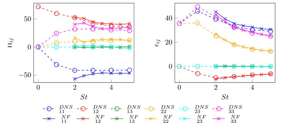
Figure 3. Pressure-strain correlation (left) and dissipation (right) over normalized time.
