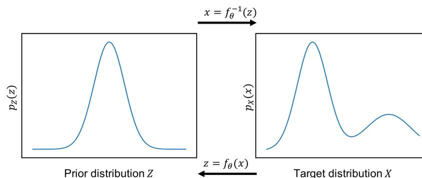
Figure 1. Change of variables. The bijective function  $f_\theta^{-1}$  transforms the prior distribution to the target distribution.
