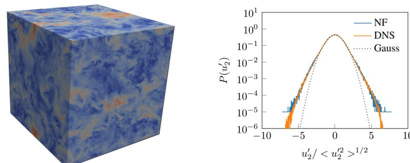
Figure 2. Left: Snapshot of a turbulent velocity field from HST. Right: PDF of the  $u'_2$  velocity showing non-Gaussian behavior.
