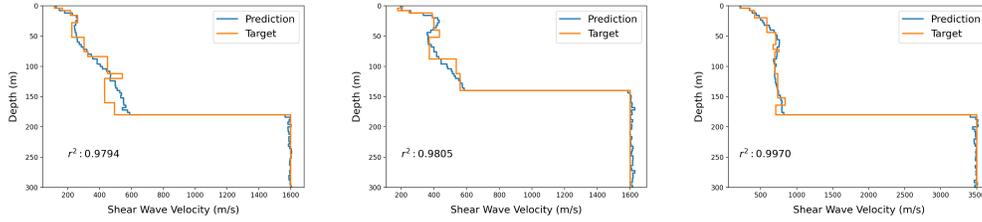
Figure 4: Three randomly chosen examples from test dataset. Each figure shows the true output "Target" and the prediction of DNN.
