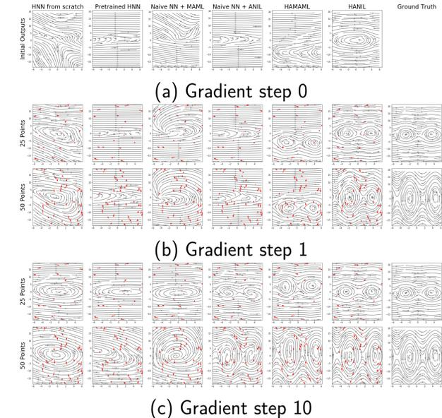
Figure: Predicted vector fields (gray streamlines) by adapting the learners to observations of new pendulum systems as given point dynamics (red arrows) after the corresponding gradient steps.
