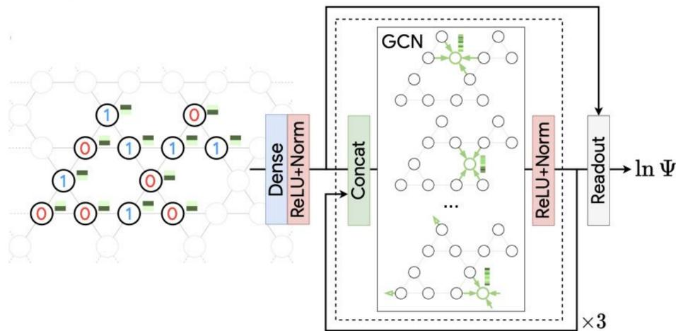
Graph neural networks can contain the inductive bias of capturing arbitrary geometries. We use a special kind of GNN, graph convolutional network, as the GNA:
