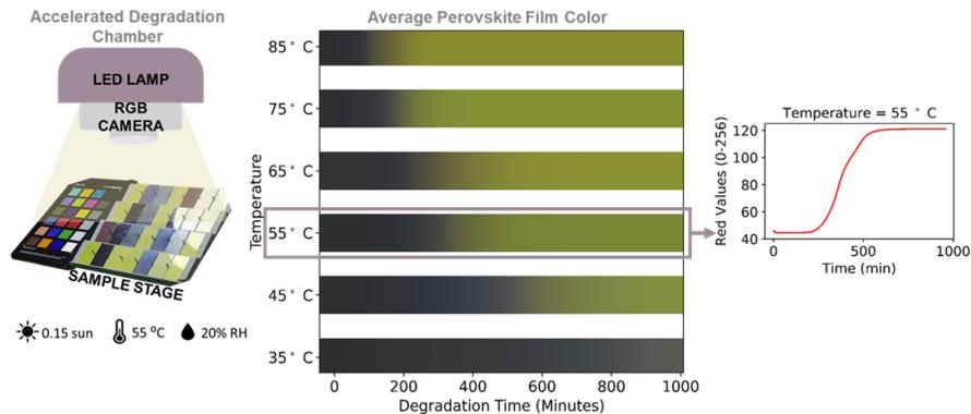
Figure 1: The experimental process. a) A schematic diagram of the in-house accelerated degradation chamber with a superimposed camera image of degrading MAPI films. b) Average perovskite film color as a function of time at different temperatures. c) Processed average red color component as a function of time for films degraded at  $T = 55\text{ }^{\circ}\text{C}$ .
