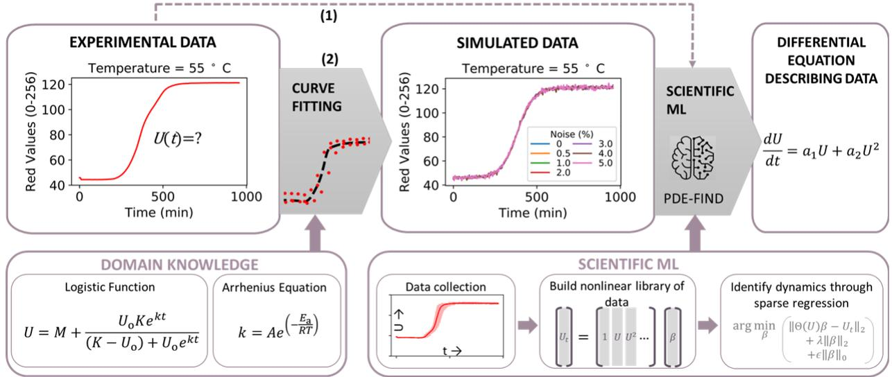
Figure 2: Schematic diagram of the data-management workflow used in this study. Workflow (1) involves the application of PDE-FIND to experimental data; Workflow (2) first fits the experimental data to create a simulated dataset, optionally adds Gaussian noise, then applies PDE-FIND
