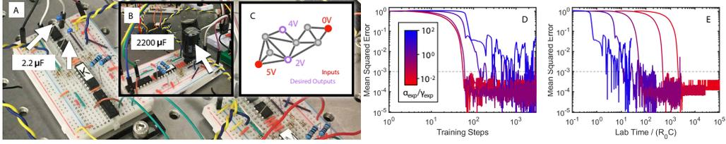
Figure 1: Out of equilibrium learning in a physical network. (A) A single edge (in both free and clamped networks) with parallel  $2.2\mu\text{F}$  capacitors highlighted with arrows. (B) A single edge with a parallel  $2200\mu\text{F}$  capacitors. (C) Network structure with inputs and outputs for the allosteric task used in (D)-(E). Typical error traces for an allosteric task as a function of training steps (D) and relaxation times (E). Colors indicate ratio of learning to relaxation rates.
