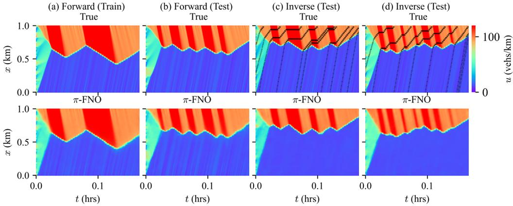
Figure 3: Comparison of true and  $\pi$ -FNO predicted solutions. Sub-figure (a) is a training scenario, and (b)-(d) are test scenarios. The dotted curve is the input locations of  $\bar{u}_b$  for the inverse problem.
