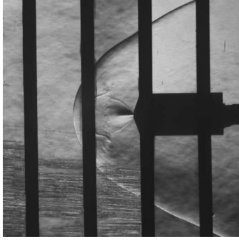
Figure 1: Schlieren image data of rocket (horizontal black rectangle) with visible exhaust plume thrusting against supersonic freestream flow. The bow shock is the curved edge that spans figure from top to bottom.
