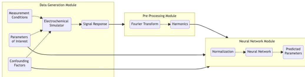
Figure 1: Detailed schematic of Phase 1 or pre-training phase - contains data generation module, physics-based processing module and a deep learning module.
