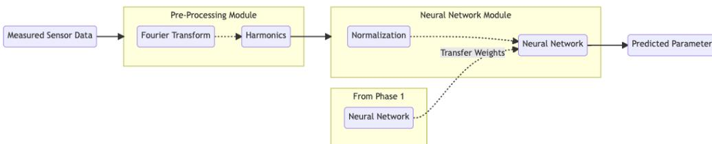
Figure 2: Detailed schematic of Phase 2 or fine-tuning phase demonstrating parameter estimation from measured sensor data - contains measured sensor data, physics-based processing module, and a deep learning module with network weights initialized from Phase 1.
