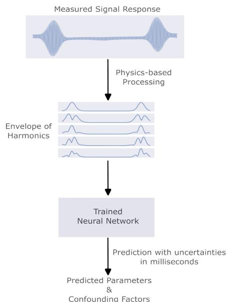
Figure 4: Schematic demonstration of the analysis workflow during prediction phase.
