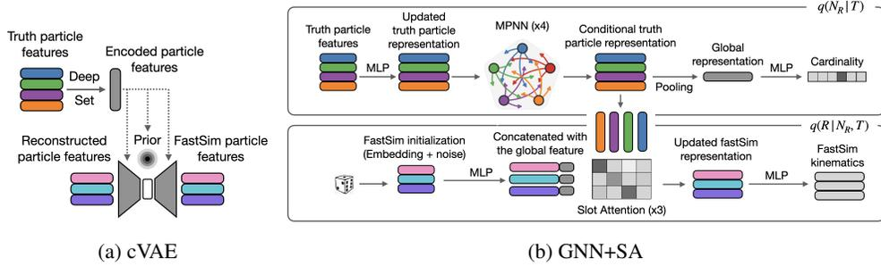
Figure 1: Architectures of the two models
