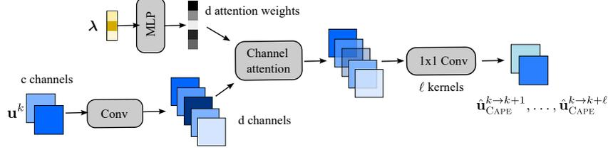
Figure 2: The CAPE module for one type of convolution (residual connections are omitted).
