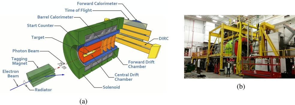
Figure 1: The GlueX detector system. (a) Schematic of the GlueX spectrometer with labels for most of the major detector systems. (b) The GlueX Spectrometer at Jefferson Lab with a human in front for scale.
