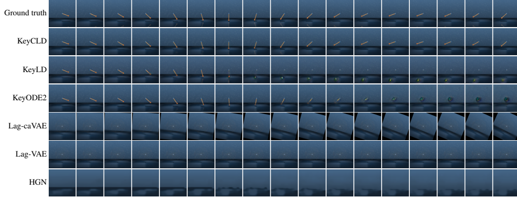
Figure 14: Future frame predictions of the unactuated pendulum. These correspond to the first row in Table 1. 50 frames are predicted based on the first three frames of the ground truth sequence to estimate the velocity. Every third frame of every sequence is shown. KeyCLD is capable of making accurate long-term predictions with minimal drift of the dynamics. Without constraint function, KeyLD is not capable of making long-term predictions. Similarly, KeyODE2 is unable of making long-term predictions. Lag-caVAE is fundamentally incapable of modelling data with background information, since the reconstructed images are explicitly rotated. Lag-VAE does not succeed in modelling moving parts in the data, and simply learns to predict static images. HGN also does not capture the dynamics and only learns the background.
