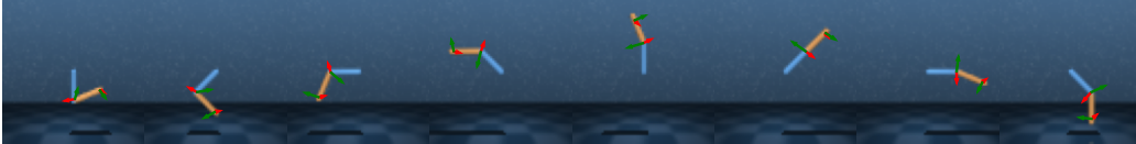
Figure 13: Visualization of the input matrix of the trained KeyCLD model of the acrobot environment. This environment has two inputs, two torques acting on each pole. The torques are modelled with opposite forces on each end of the poles, such that the residual force can be zero.
