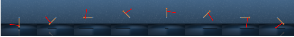
Figure 11: Visualization of the input matrix of the trained KeyCLD model of the pendulum environment. The input of this environment is a torque acting on the pendulum. In the KeyCLD framework this is correctly modelled with a force acting perpendicular on the pendulum.
