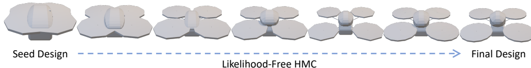
Figure 2: Sub-sampled quadcopter designs taken along the likelihood-free HMC chain using DNRE. The initial seed design on the far left has multiple structural interferences, including sensors that cut through the fuselage. As we move along the chain we see the design morph into our desired structure with very few interferences. This is achieved through increasing the arm length and changing the shape of the fuselage, as well as varying the placement of the interior sensing components.
