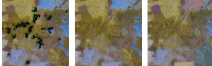
Figure 1: Metallographic textures (from left): Zoomed metallography with impurities; Removed impurities using deep inpainting; and failed semantic segmentation with Segment Anything [29].
