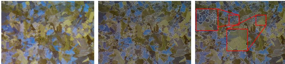
(a) Metallographic input image. (b) Supervised GB SS. (c) Wrong predictions (magnified).
